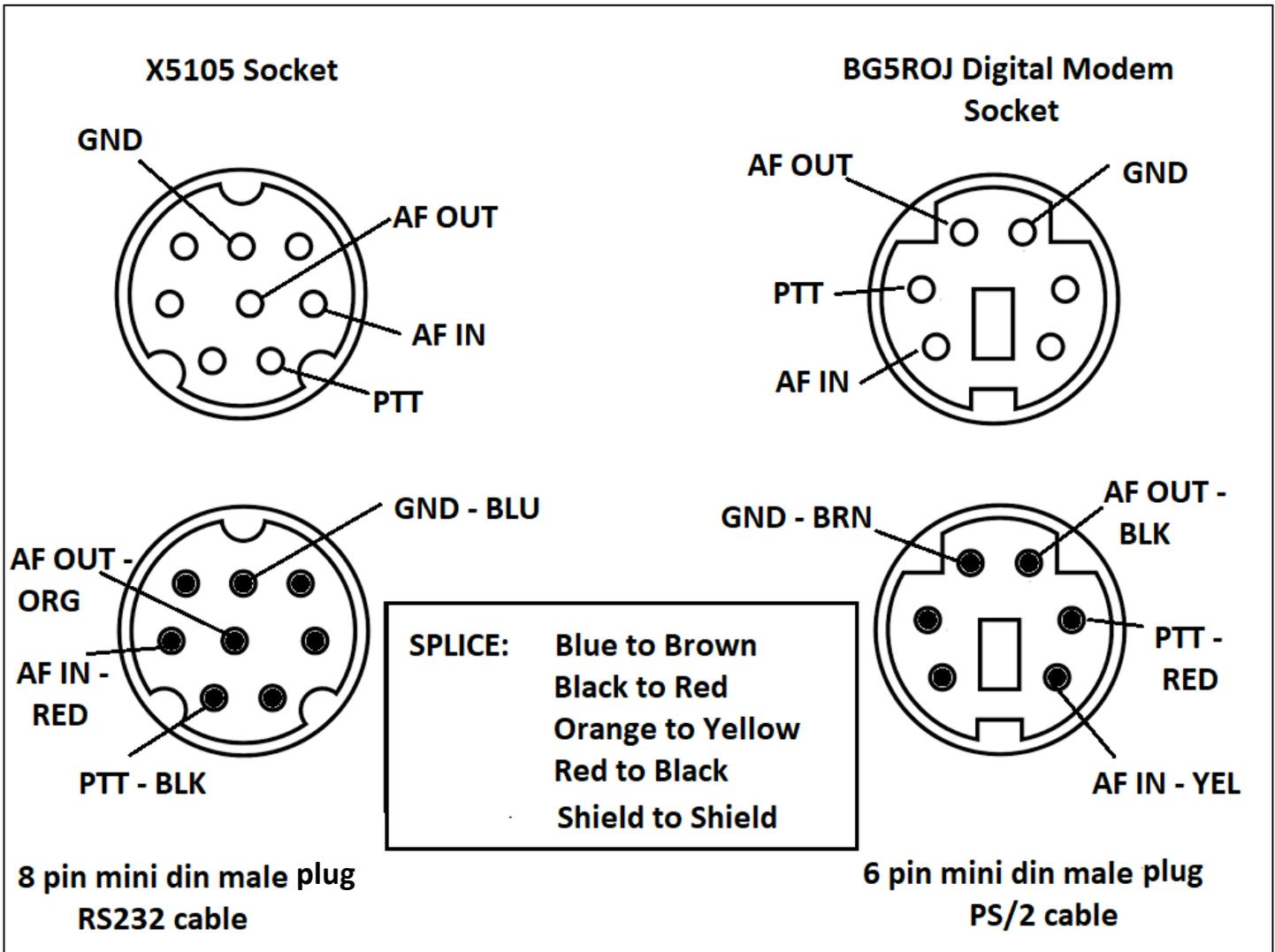
Figure 1. Modem cable splice
